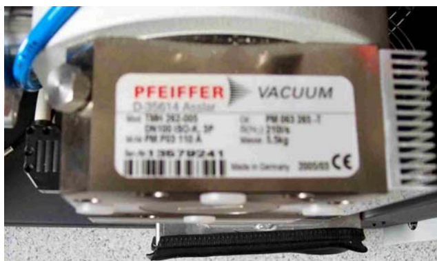
Figure 7-15. Heat Sinks Mounted on Analyzer Turbomolecular Pumps
