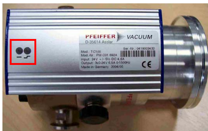
Figure 7-14. LEDs at Bottom Side of Turbomolecular Pump
