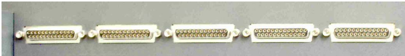
Figure 2-50. SUB D Connectors without Peripheral
