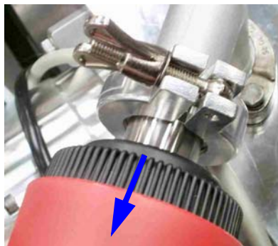
Figure 7-27. Pulling Away Electronics Cylinder of Penning Gauge
