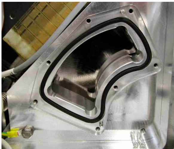
Figure 5-20. View into Analyzer - One Magnetic Coil Dismantled
