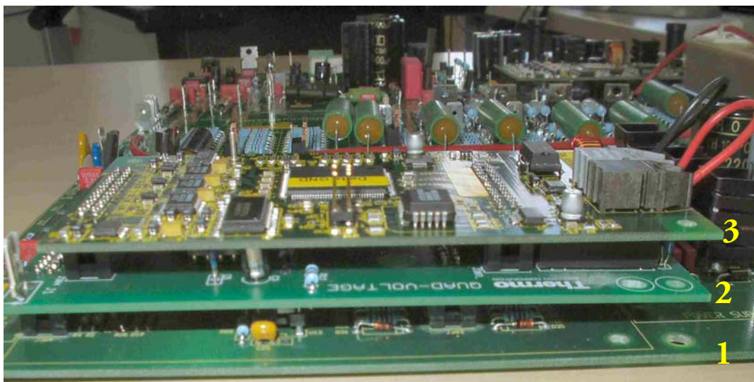
Figure 2-61. Arrangement of Focus Quad Power Supply Board
