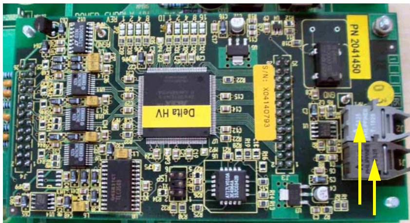
Figure 2-59. Bus Control Board (High Voltage)
