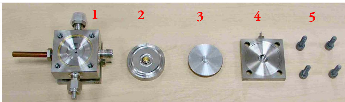
Figure 4-4. Parts of Dual Inlet System Valve
