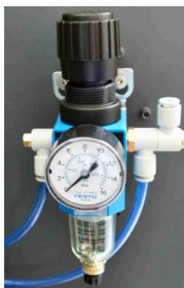
Figure 2-30. Pressure Reducer for Compressed Air - Front View
