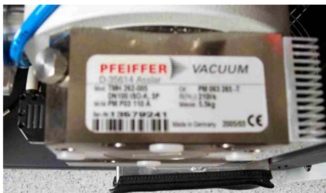
Figure 7-15. Heat Sinks Mounted on Analyzer Turbomolecular Pumps
