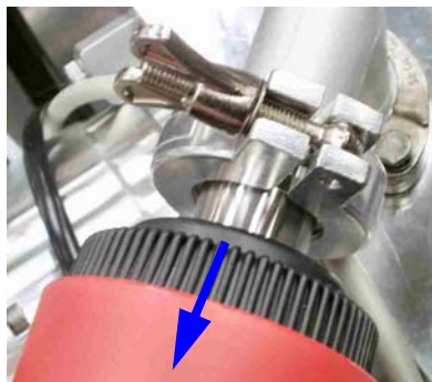
Figure 7-27. Pulling Away Electronics Cylinder of Penning Gauge
