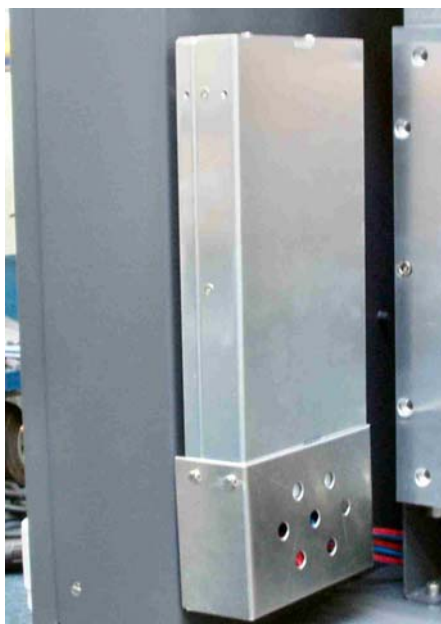
Figure 2-36. 24 V Power Supply
