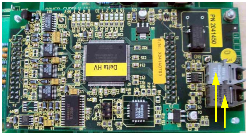
Figure 2-59. Bus Control Board (High Voltage)
