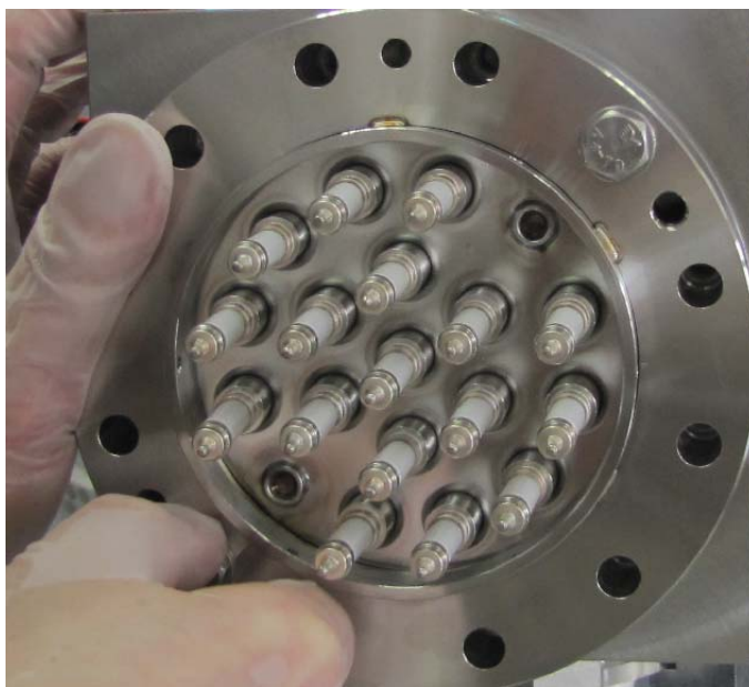
Figure 8-5. Tightening the ion source in the analyzer head
