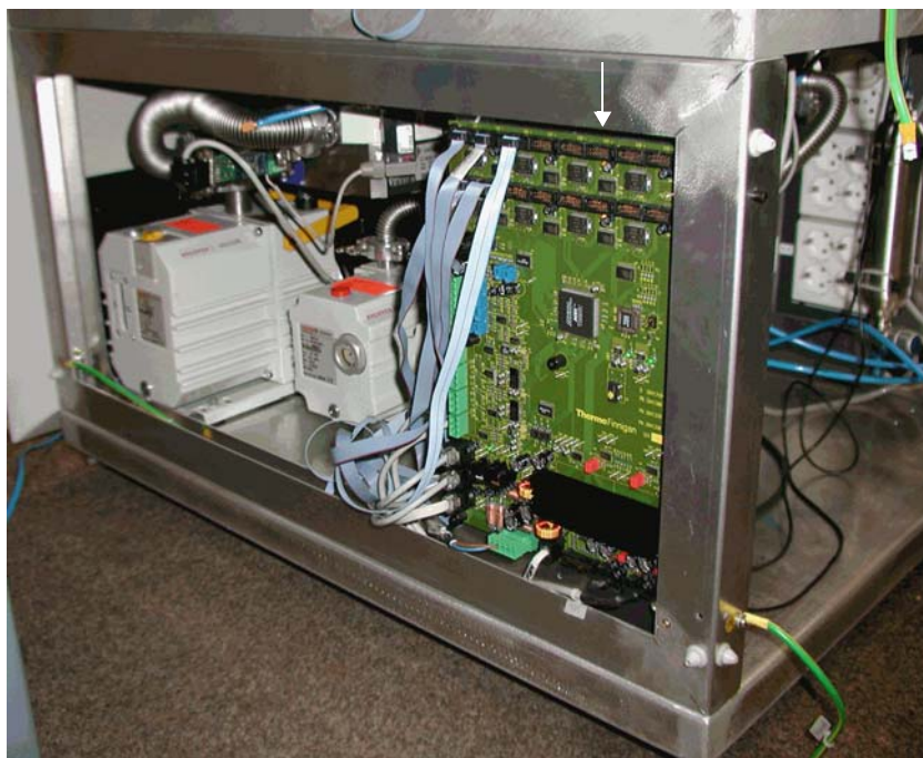
Figure 5-5. Driver board with distributor function
