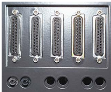
Figure 1-16. SUB D ports at rear panel of IRMS
