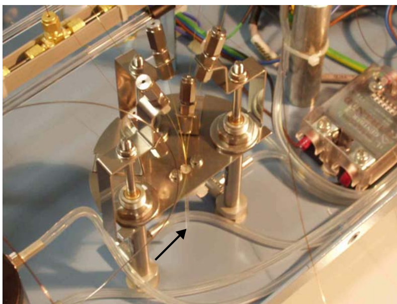
Figure 2-48. Reference inlet (open split)
