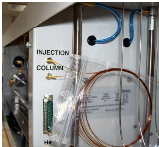
Figure 6-21. PreCon inlet and outlet connections
