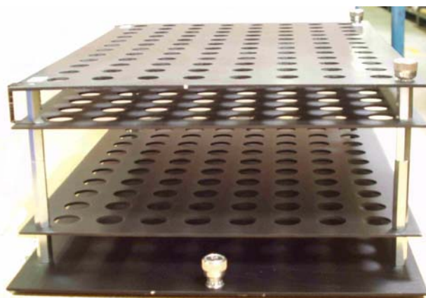
Figure 2-12. Non-thermostated sample tray - side view
